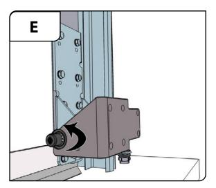
E. While the door is supported and there is no tension in the lifting cables, check if the roller moves freely into the track and also verify, by removing the bolt or nail in the rotating module, if it rotates freely until the blade reaches the track. After checking replace the nail or bolt!
