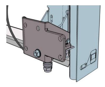
Use bolt and nut 14022 and 14023 to mount 25446 to the rotating bracket.
