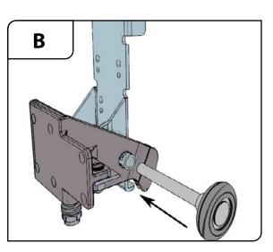
B. Insert a roller into the tube. The black rubber cap has a transportation purpose only. It may be removed when assembling the roller on the device.
